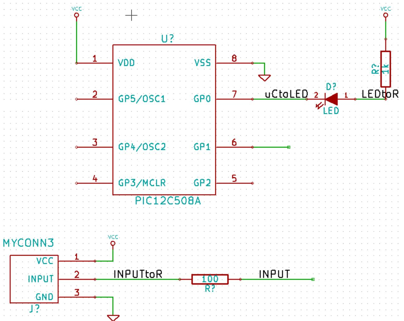
93. The program checks for wiring errors. Any wires that are not connected may generate a warning. To avoid these warnings you can instruct the program that the unconnected wires are deliberate.
