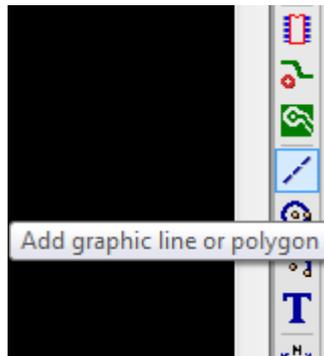
160. Trace around the edge of the board, clicking at each corner, and remember to leave a small gap between the edge of the green and the edge of the PCB.
