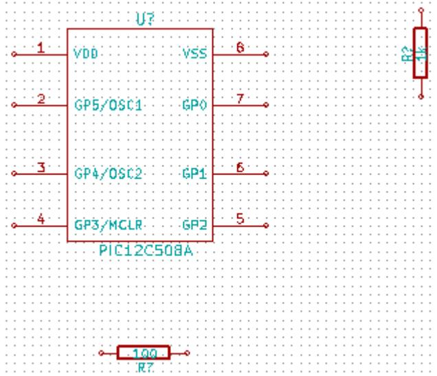
40. Hover the mouse over the microcontroller component. Press 'y' and 'x' on the keyboard. Notice how the component is mirrored on its x and y axes. Press 'y' and 'x' again to return it to its original orientation.
