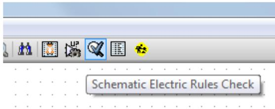
102. This will generate a report to inform you of any errors or warnings such as wires being disconnected. You should have 0 Errors and 0 Warnings. A small green arrow will appear in the location of the error if you have made a mistake. Check “Write erc report” and press the “Test ERC” button again to receive more information about the errors.
