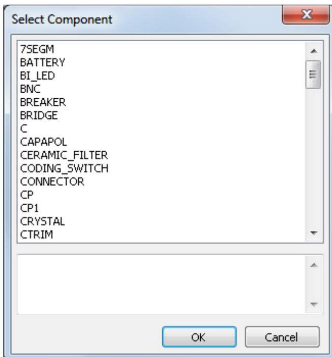
20. Scroll down and double click on “R”. This will close the “Select Component” dialog and place component “R” onto your schema.
