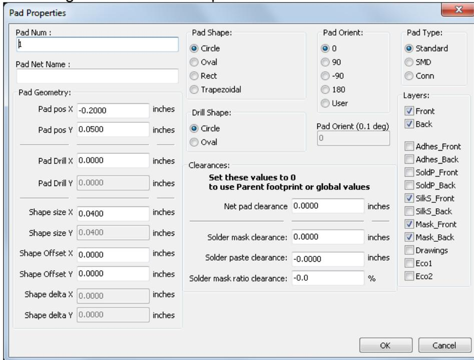
194. Set the “Pad Num” to “1”, “Pad Shape” to “Rect”, “Pad Type” to “SMD”, “Shape Size X” to “0.4”, and “Shape Size Y” to “0.8”. Click “OK”.
