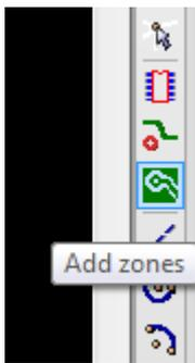
153. We’re going to trace a rectangle around the board, so click where you want one of the corners to be. In the dialog that appears, set “Pad in Zone:” to “Thermal relief” and “Zone edges orient:” to “H,V”, and then click “OK”.
