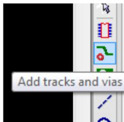
145. Click in the middle of pin 1 of “J1” and run a track to the pad “R2”. Double-click to set the track’s end point.
